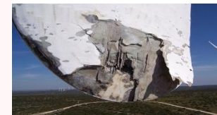
Blade Tip Damaged by Lighting Strike
